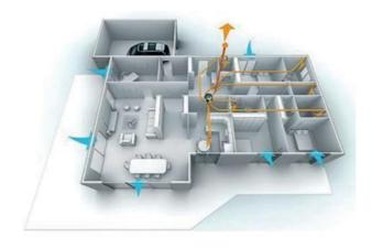
Their functioning this based in the principle of sweeping the air inside the houses from the dry rooms (bedrooms and living room) to the wet rooms (kitchen and bathrooms).
